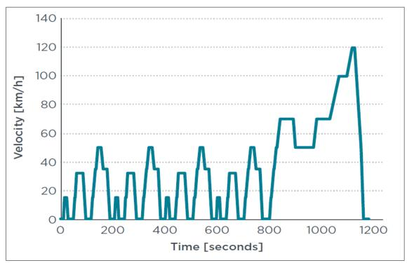
Figure 5: NEDC according to Directive 70/220/EEC, source: (ICCT 2014b)
