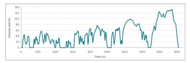
Figure 11: WLTP test cycle (WLTC), Source: (ICCT 2014b)
