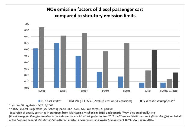
Figure 23: NO<sub>x</sub> emission factors of diesel passenger cars-statutory limits vs real-world emissions
