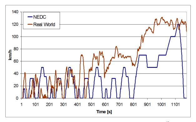
Figure 8: Type approval testing passenger cars compared to real-world driving (CADC)<sup>12</sup>
